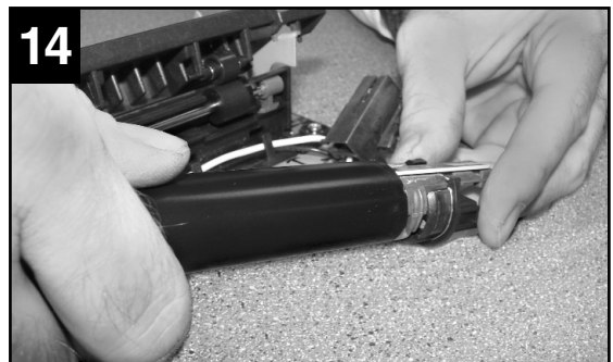
14 Slide the film onto heating element, turning film a few times to make sure grease is evenly spread on inner surface of replacement film.
