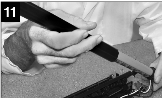
11 Carefully slide used fixing film off end of the heater assembly.
